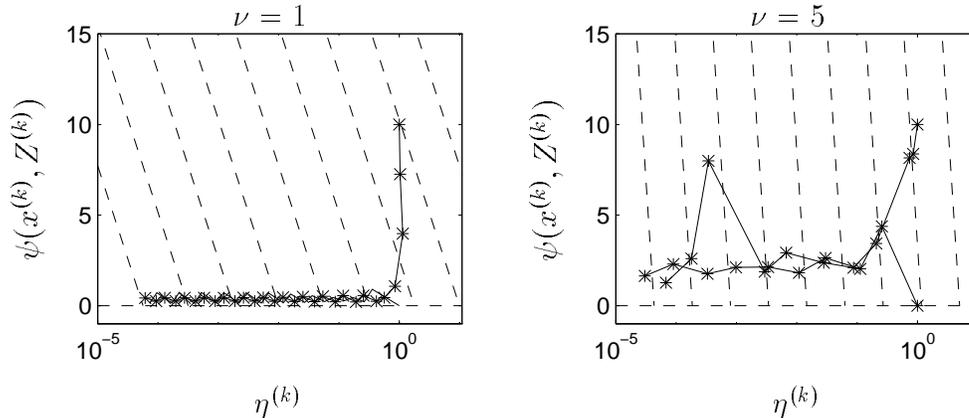
**Figure 10:** Trajectories of the duality gap  $\eta$  and the deviation from centrality  $\psi$ , for  $\nu = 1$  (at left) and  $\nu = 5$  (at right), with two different starting points. The first starting point lies on the central path ( $\psi = 0$ ); the second point lies at  $\psi = 10$ . The dashed lines are level curves of the primal-dual potential function  $\varphi$ .
