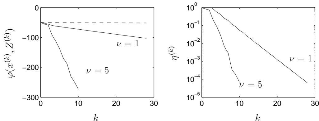
**Figure 9:** The potential function  $\varphi$  and the duality gap  $\eta$  versus the iteration number  $k$ , for two values of  $\nu$ . The problem is a matrix norm minimization problem with 10 matrices in  $\mathbf{R}^{10 \times 10}$ . The dashed line in the left-hand plot shows the upper bound given by Theorem 5, *i.e.*, a reduction of 0.05 per iteration.
