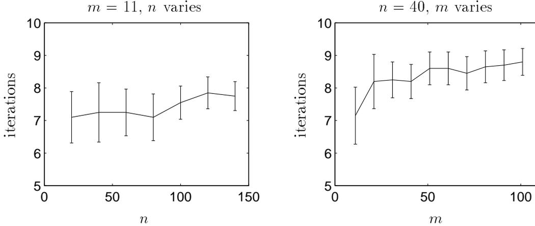
**Figure 12:** The average number of iterations to solve the matrix norm minimization problem with  $k$  matrices in  $\mathbf{R}^{p \times p}$ , which yields a semidefinite program of dimension  $m = k + 1$ ,  $n = 2p$ . In the left plot  $k = 10$  ( $m = 11$ ) is fixed and we vary  $p$  ( $n$ ). In the right plot  $p = 20$  ( $n = 40$ ) is fixed and we vary  $k$  ( $m$ ). Each point is the average of 20 random instances. The error bars show the standard deviation.
