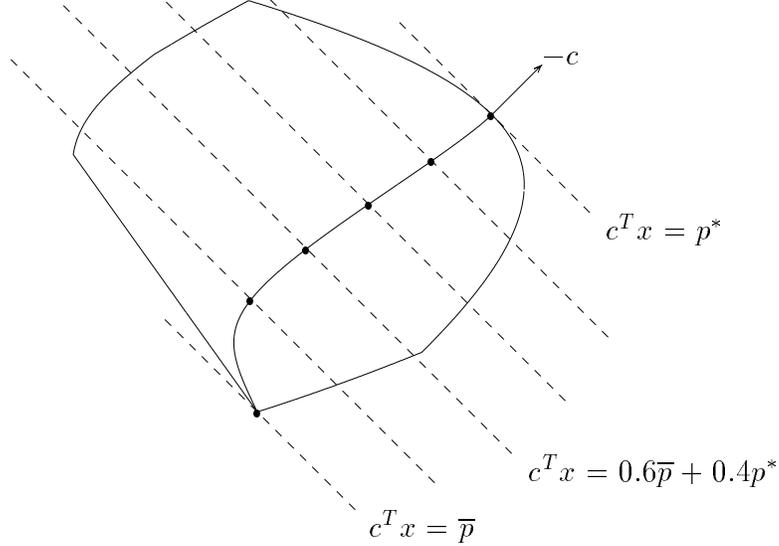
**Figure 6:** The central path for the semidefinite program of Figure 1. The dashed lines represent level sets  $c^T x = \gamma$ , for six values  $\gamma$  in the interval  $[p^*, \bar{p}]$ . The heavy dots are the analytic centers  $x^*(\gamma)$  of the linear matrix inequality (53). The central path is formed by the analytic centers  $x^*(\gamma)$  when  $\gamma$  varies between  $p^*$  and  $\bar{p}$ .
